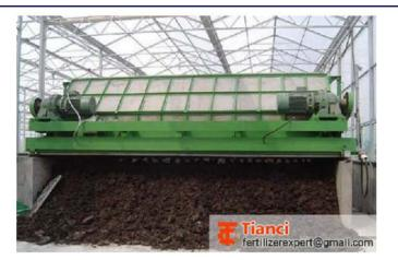
This horizontal compost turner machine is the key fertilizer equipment in organic fertilizer production machines for making organic compost fertilizer, and it is the first step. Organic fertilizer production has to be protein organic matter, so the first step has.
