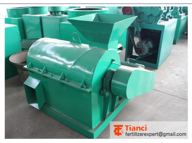
is specialized in crushing half wet material with high moisture which is a professional equipment of fibrous material crushing. With high-speed rotating blade, it features good granularity and high efficiency. It does a good effect in crushing hen manure, sodium humate in organic fertilizer production processing.
